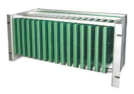
The 16-point input card layout isolates individual points from each other and from the system electronics by opto-couplers.
