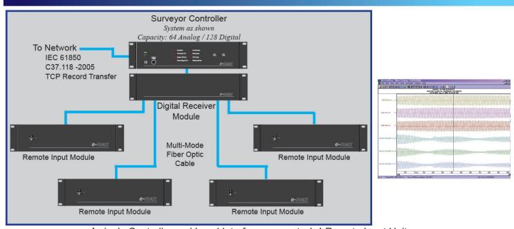
A single Controller and Local Interface connects 1-4 Remote Input Units.
